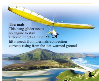
Figure 1.13 (b): A hang-glider uses thermals, rising convection currents from sun-warmed ground, for lift.
