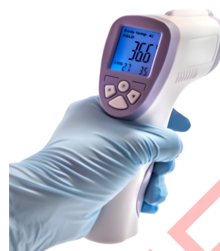
Figure 1.19: Infrared thermometer measuring body temperature without physical contact.
