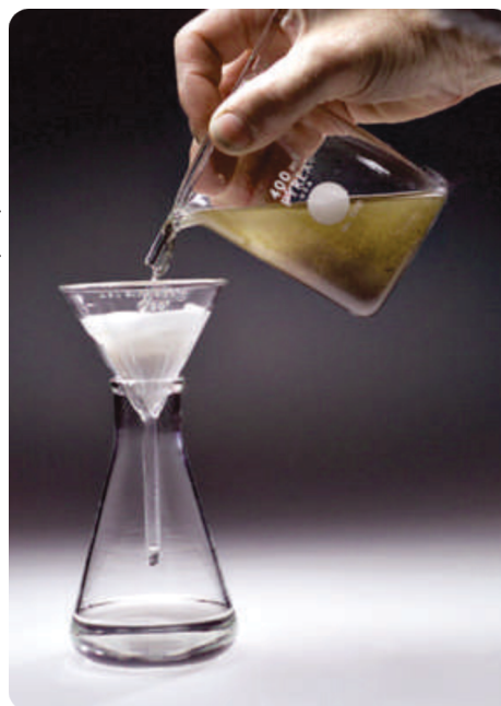
Purifying a heterogeneous mixture by filtration
