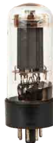
Fig. 1.2 (a) Vacuum tube
